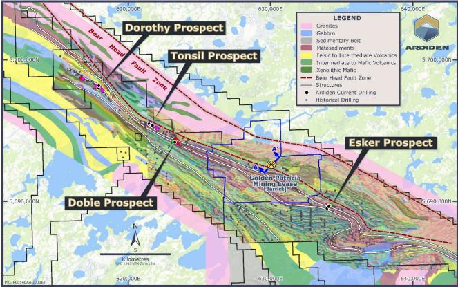
Figure 1-Drilling Locations along the Western Hub – (Cross-section line A—A' through Golden Patricia Mine shown on Figure 6)
