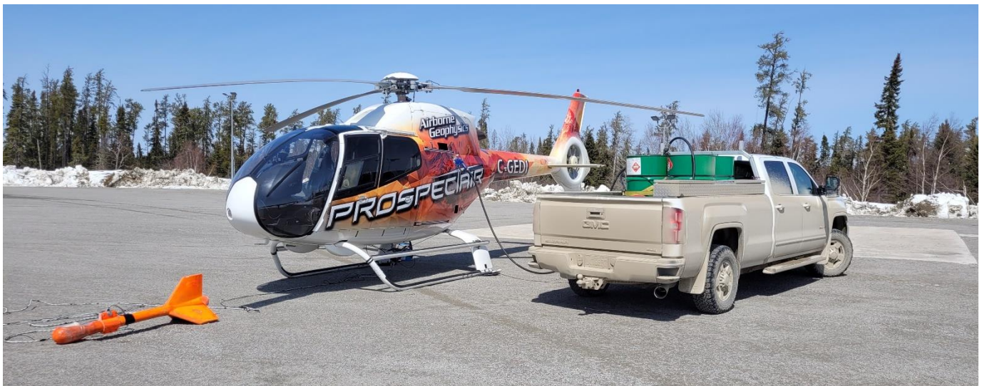
Figure 1: PROSPECTAIR's EC120 helicopter efficiently handles the equipment load and required survey range
