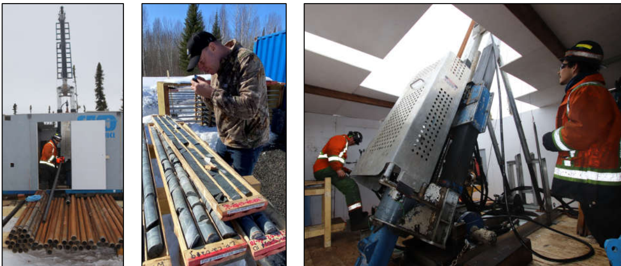
Figure 1- Ardiden's Exploration Manager, Haydn Daxter, logging drill core at the Esker Gold Prospect Drill Site
