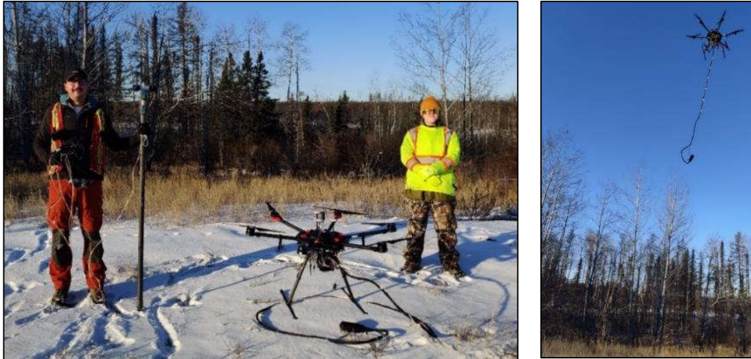
Figure 17 - UAV Magnetic Survey Equipment Setup at South Limb
