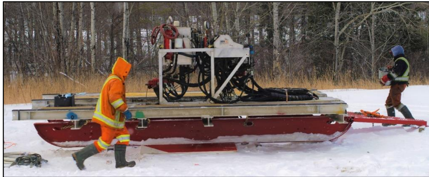
Figure 4-Drill Rig undergoing conversion to 'skid' mode for Winter ease of movement by Dozer
