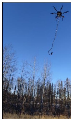
Figure 5- UAV Magnetic Survey Equipment Setup at South Limb
