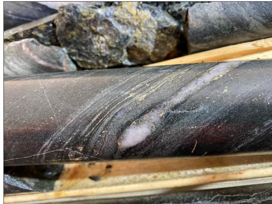
*Pyrite + Pyrrhotite associated with quartz veining in KAS20-001*
