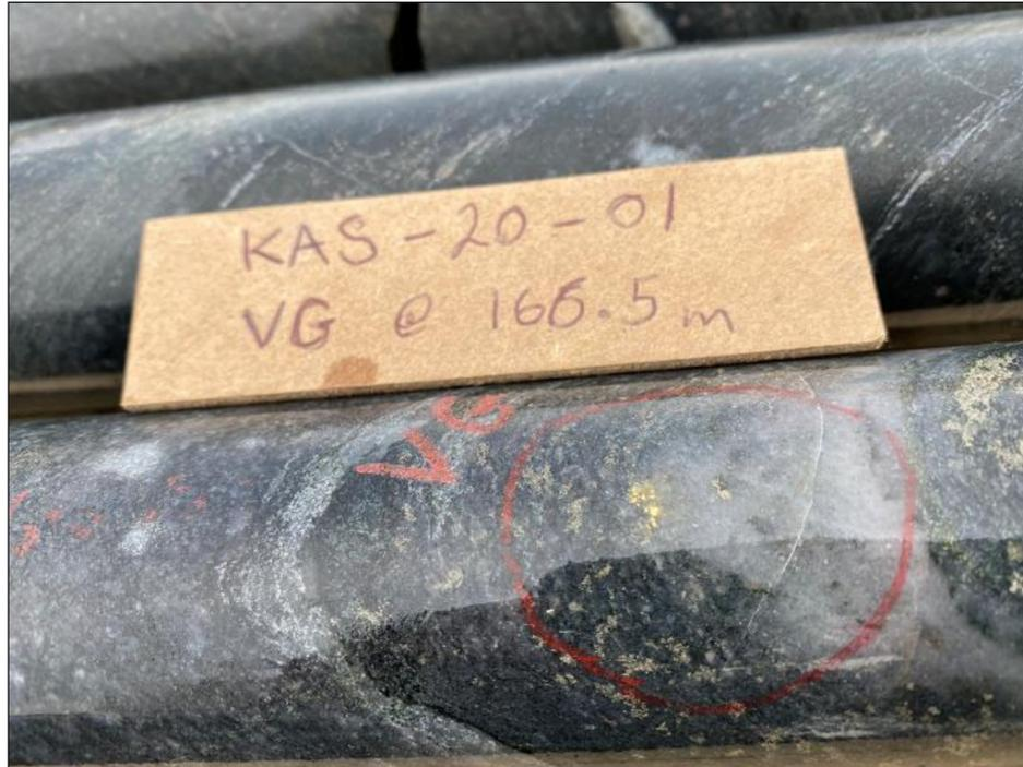
*Visible Gold logged in drillhole KAS20-001 at 166.5m*
