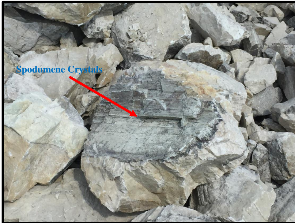
Figure 2. Bulk sample of Spodumene bearing pegmatite obtained from the North Aubry prospect. Highlighted in the image are the large high quality Spodumene crystals
