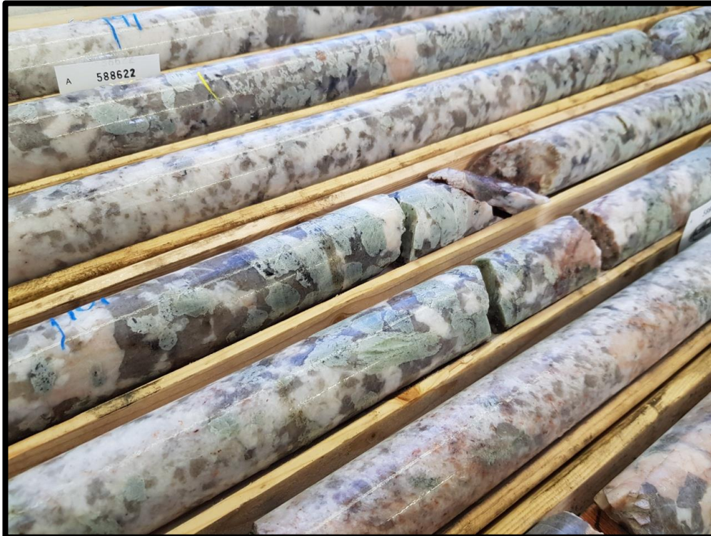
Figure 8. Image of the drill core obtained from drill hole SA-18-07, Note large pale green to whitish coarse tabular spodumene crystals with quartz and feldspar.
