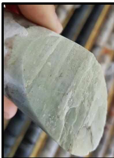
**Figure 1.** Image of drill-core (from drill-hole SA-18-07) showing a spodumene crystal.
