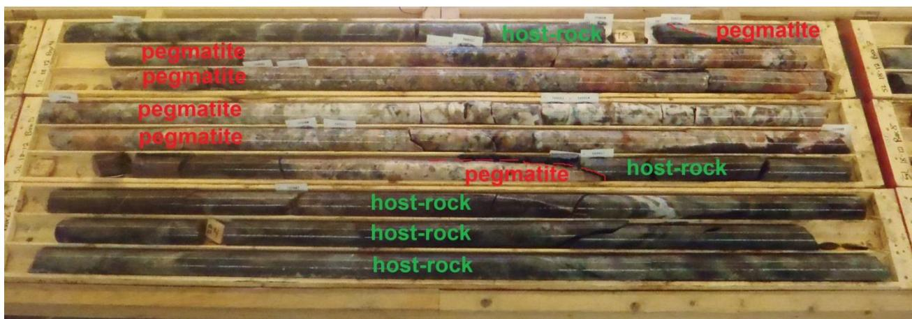
**Figure 2.** Drill core obtained from drill hole SA-18-12 showing the previously unknown pegmatite intersected from 15.00m to 21.80m; the white coloured material in the pegmatite is mostly spodumene.
