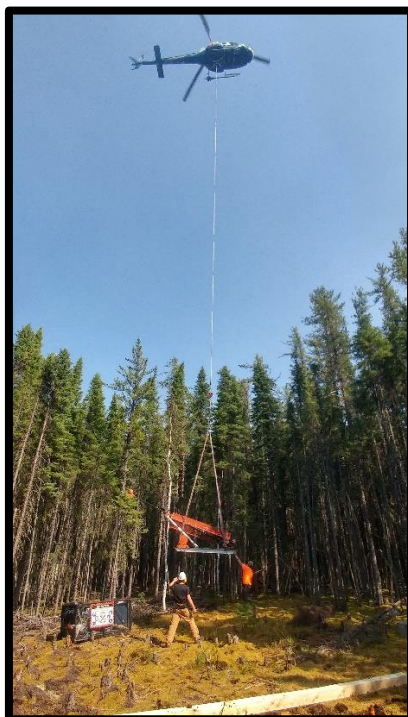
Figure 1. Image showing the helicopter airlifting drilling equipment onto the first drill pad at the Kasagiminnis Lake Property
