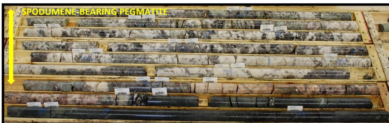
**Figure 1.** Drill core obtained from drill hole SL-17-75 (from 76.4.8m to 89.0m) showing the intersection of high-quality spodumene-bearing pegmatite (the lighter coloured material in the photo is the Pegmatite, whilst the darker material is Mafic Volcanic).
