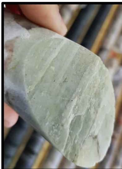
**Figure 4.** Drill core images obtained from drill hole SA-18-07 show very large high quality spodumene crystals.
