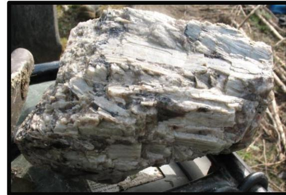
Sample of large high grade spodumene crystals exposed at North Aubry prospect, Seymour Lake, Ontario Canada.
