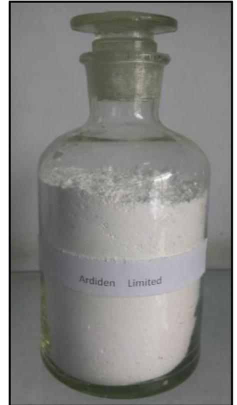
Final Lithium Carbonate ( $\text{Li}_2\text{CO}_3$ )
