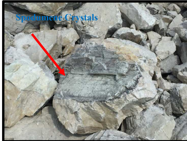
Figure 4. Bulk sample of Spodumene bearing pegmatite obtained from the North Aubry prospect.
