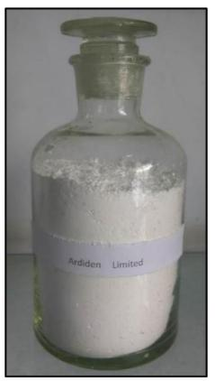
Final Lithium Carbonate (Li<sub>2</sub>CO<sub>3</sub>) Products of Battery Level
