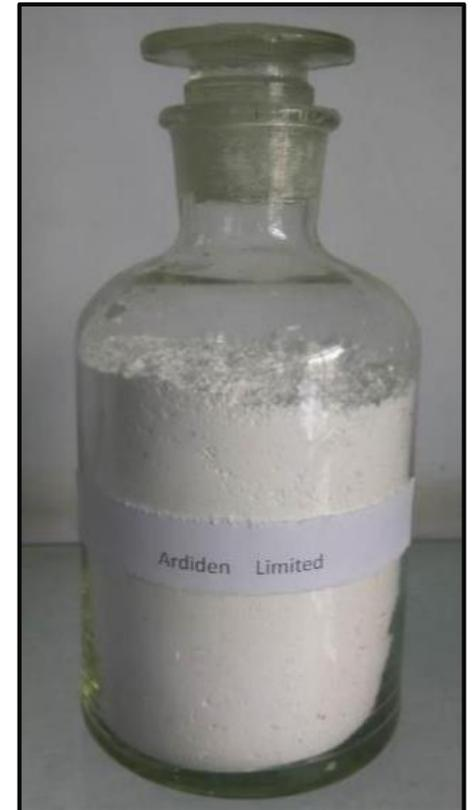
Final Lithium Carbonate ( $\text{Li}_2\text{CO}_3$ )
