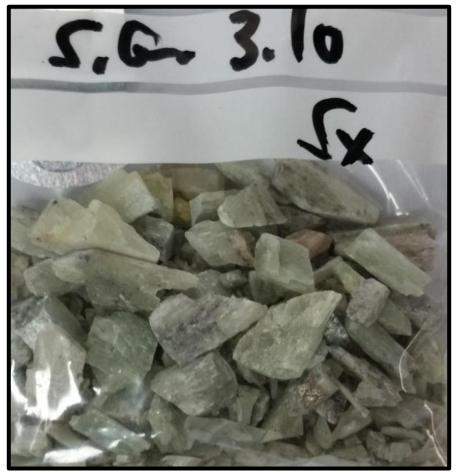
Figure 10. Sample of coarse lithium concentrate (Spodumene) created with DMS at the specific gravity of 3.10. IMO also noted the significant presence of micas in the spodumene concentrate sample at the coarse crushing size of 9.5mm. Ardiden will undertake additional testwork on the micas to better understanding of the material and whether this material could improve the Li<sub>2</sub>O recovery and concentrate grade.
