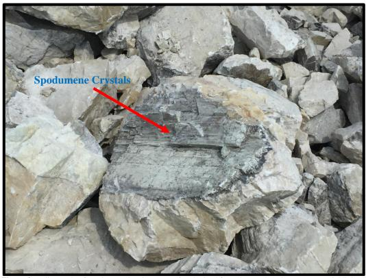
**Figure 3.** Bulk sample of spodumene-bearing pegmatite obtained from the North Aubry prospect. Highlighted in the image are the large high quality spodumene crystals.
