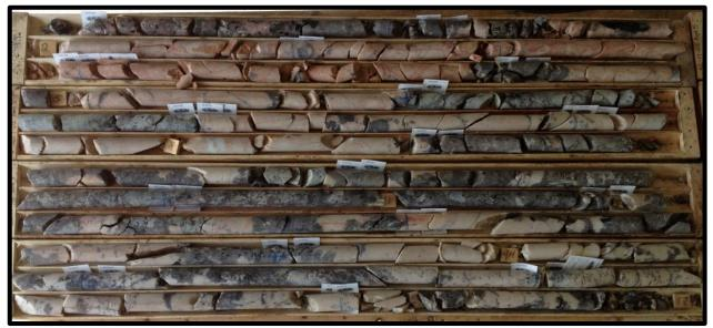
Figure 8. Drill core from diamond drill hole SL-17-02 showing high quality spodumene mineralisation from 0m to 17m.
