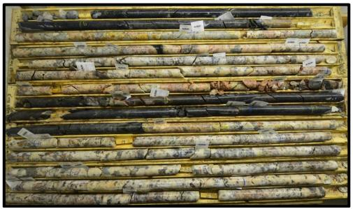
**Figure 5.** Drill core obtained from hole SL-16-68 showing a portion of the 16m intersection of high quality spodumene-bearing pegmatite.
