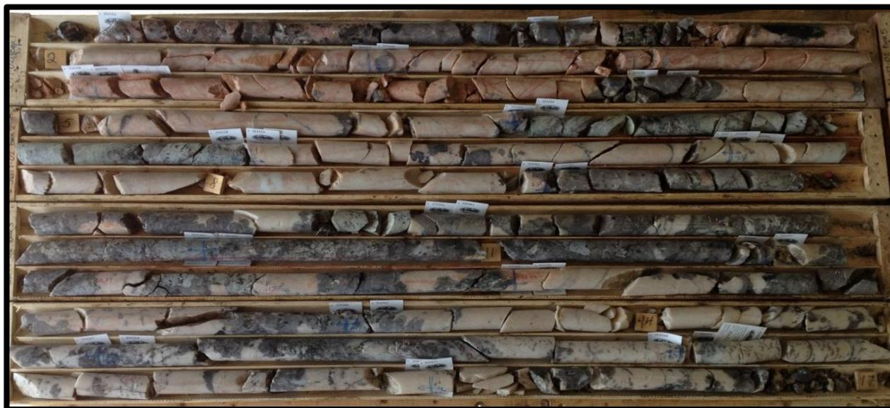
**Figure 8.** Drill core from diamond drill hole SL-17-02 showing high quality spodumene mineralisation from 0m to 17m.
