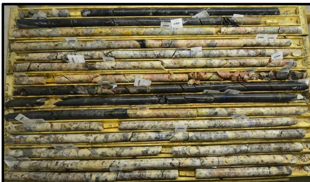
**Figure 5.** Drill core obtained from hole SL-16-68 showing a portion of the 16m intersection of high quality spodumene-bearing pegmatite.
