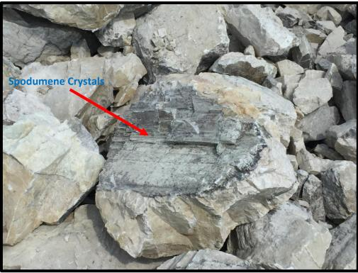
Figure 9. Bulk sample of Spodumene bearing pegmatite obtained from the North Aubry prospect. Highlighted in the image are the large high quality Spodumene crystals.
