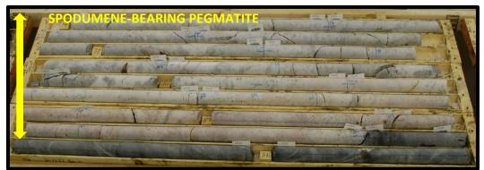
**Figure 6.** Drill core obtained from drill hole SL-17-37 showing the intersection of high-quality spodumene-bearing pegmatite (the lighter coloured material in the photo is the pegmatite, whilst the darker material is mafic volcanic).
