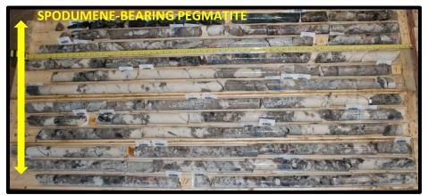
Figure 3. Drill core from diamond drill hole SL-17-03 showing high quality spodumene mineralisation from 3m to 19m (the lighter coloured material in the photo is the pegmatite, whilst the darker material is mafic volcanic).
