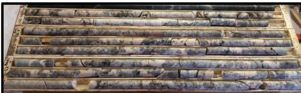
Figure 2. Drill core obtained from drill hole SL-16-62 showing the 11.5m intersection of high quality spodumene-bearing pegmatite.
