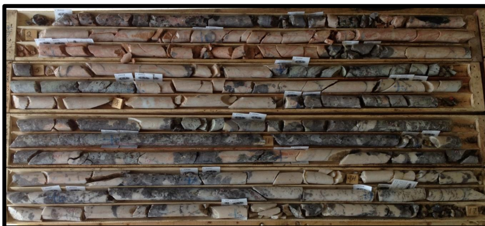
Figure 6. Drill core from diamond drill hole SL-17-02 showing high quality spodumene mineralisation from 0m to 17m.
