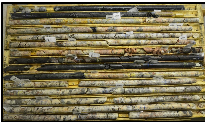
Figure 3. Drill core obtained from hole SL-16-68 showing a portion of the 16m intersection of high quality spodumene-bearing pegmatite.
