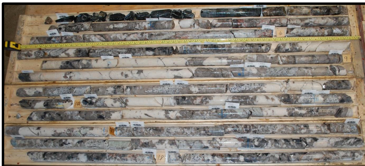
Figure 1. Drill core from diamond drill hole SL-17-03 showing high quality spodumene mineralisation from 3m to 19m.
