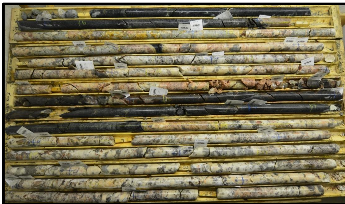
Figure 2. Drill core obtained from hole SL-16-68 showing a portion of the 16m intersection of high quality spodumene-bearing pegmatite.
