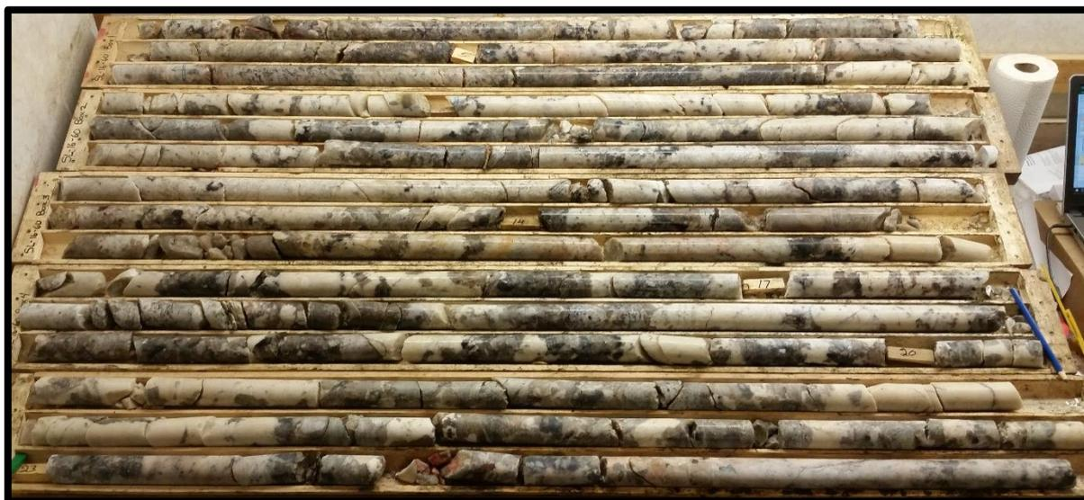
**Figure 2.** Drill core obtained from hole SL-16-60 showing a portion of the 23.5m intersection of high quality spodumene-bearing pegmatite.
