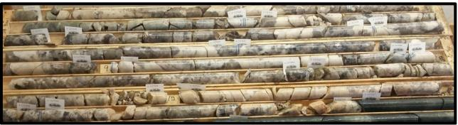
Figure 1. Drill core obtained from drill hole SL-16-58 showing the 12.2m intersection of high quality spodumene-bearing pegmatite.
