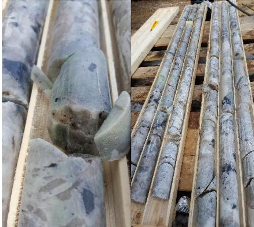
**Figure3.** Drill core from the due diligence drilling at the Seymour Lake Project showing multiple intersections of spodumene mineralisation in the pegmatite structures.
