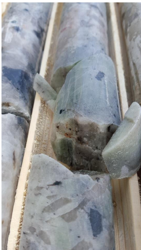
Figure 1. Drill core from the Seymour Lake Project showing multiple intersections of spodumene mineralisation in the pegmatite structures.
