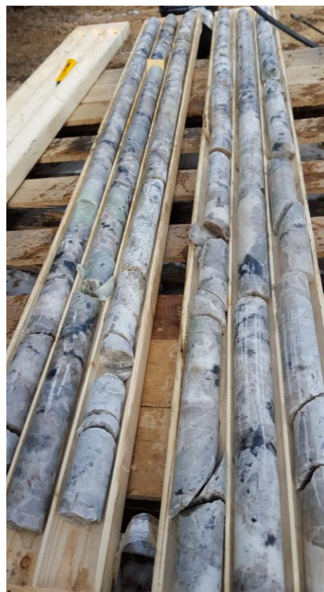
Figure 1. Drill core from the Seymour Lake Project showing multiple intersections of spodumene mineralisation in the pegmatite structures.
