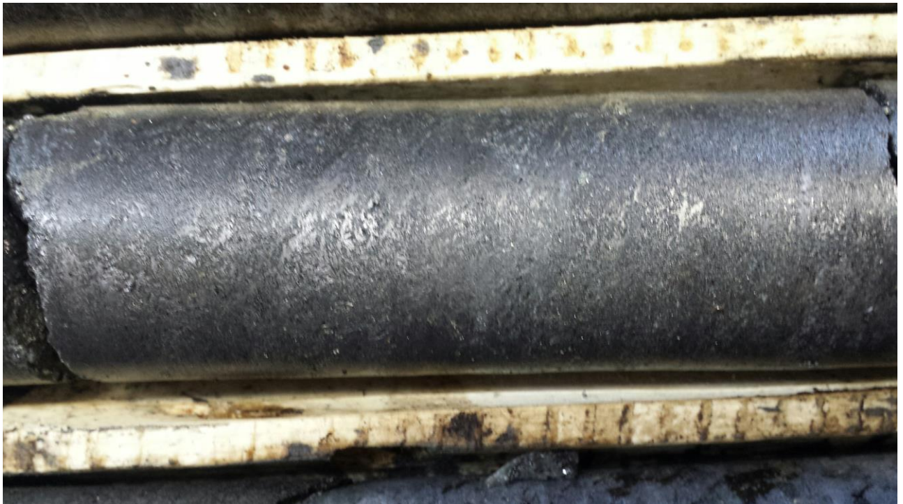
Figure 12: Graphite core from drilling at Manitouwadge graphite project in Ontario, Canada (Hole EM 12-05 at Silver Star Prospect)
